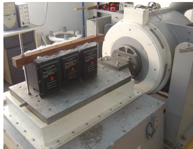
VIBRATION TEST- HORIZONTAL
